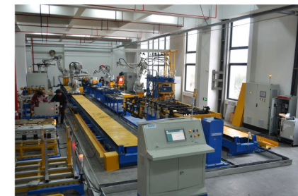
Fully automatic ring main unit welding production line
