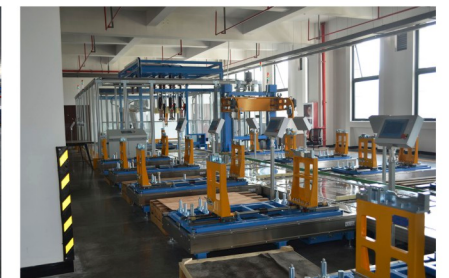
Outdoor circuit breaker intelligent production line
