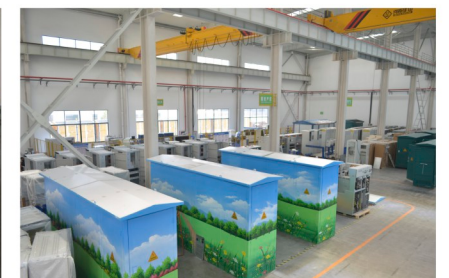
Prefabricated substation workshop
